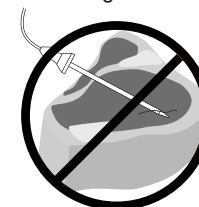
(Figure C) Incorrect placement of probe
