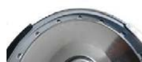
Gasket wrong position
